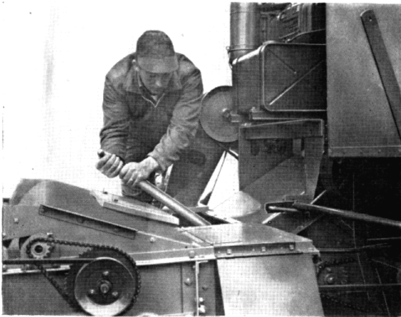
Fig. 30 Straightening Cylinder Teeth
